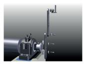
The Offset Fixtures' laser is adjustable in a plane parallel to the flange face of the stationary machine and can be set at any position to eliminate the offset from the driven unit.
