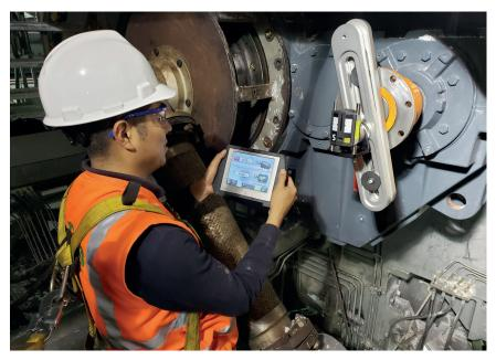
Machines with offset drives are often thought of as insensitive to alignment errors between driving and driven shaft. However, they cannot absorb angular misalignment between the shafts, hence our kit the Offset Fixtures. The fixture kit, consisting of machined parts with high precision (parallelity and flatness within 0,03 mm) makes it possible to do accurate alignment which conventional methods can't do.
