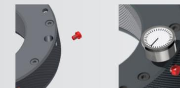
**d** Activate the pump until you reach the desired displacement of the HMV (value of displacement available on our NTN-SNR catalogue).
